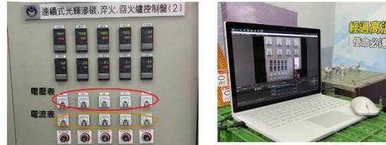
Figure 9 The current and voltage video monitoring diagram of the temperature rise measurement experiment in the furnace
