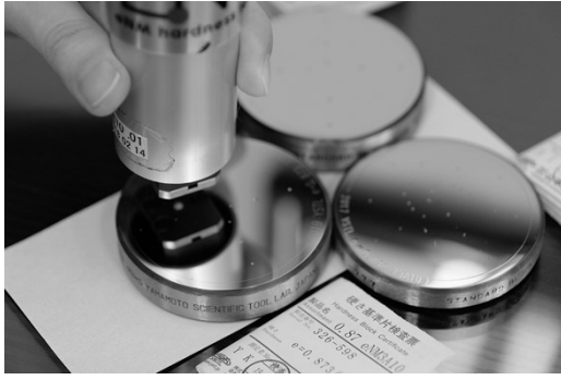
Figure 2 Hardness reference blocks e = 0.87, 0.63 and 0.19
