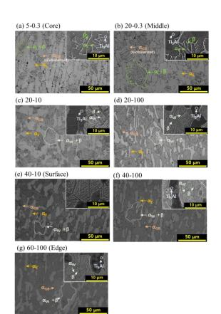
**Figure 3**. OM and SEM microstructures of STA heat treated samples with different solution treatment conditions of (a) 5-0.3, (b) 20-0.3, (c) 20-10, (d) 20-100, (e) 40-10, (f) 40-100, (g) 60-100.
