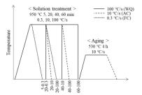
Figure 1. STA heat treatment conditions used in this study.
