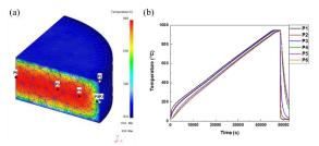
Figure 2. (a) Heat transfer analysis during solution treatment of the approximate size of an aero-engine disk of Ti64 and (b)  $P1\sim P6$  point tracking during solution treatment.
