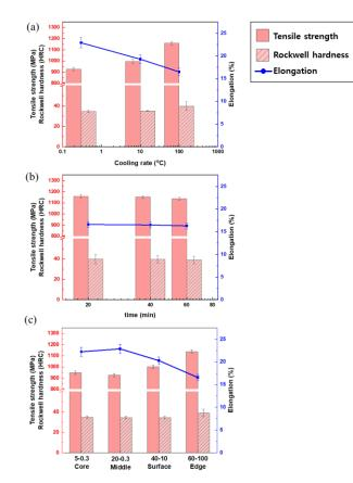
**Figure 4**. Changes of Rockwell hardness and tensile properties (tensile strength and elongation) at the room temperature according to (a) holding time, (b) cooling rate, and (c) thermal history of area.
